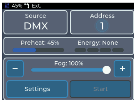
Fig. 1: Main menu - Boa 64 when heating up
